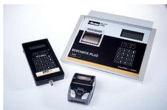
**Figure 6** – Integrity test instruments can measure pressure decay with millibar sensitivity and convert to diffusional flow. They are available with different degrees of functionality with some that can carry out a fully automated integrity test
